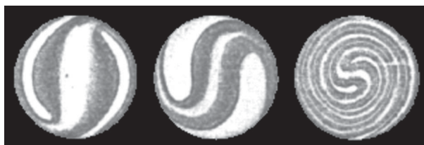
Figure 1. Drawings by Lehmann of droplet textures that wind and rotate under the action of an increasing temperature gradient (from left to right) (adapted from Ref. [10]).
